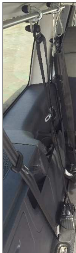
Figure 17 – Wheelchair occupant seat belt slider bar adjustment.
