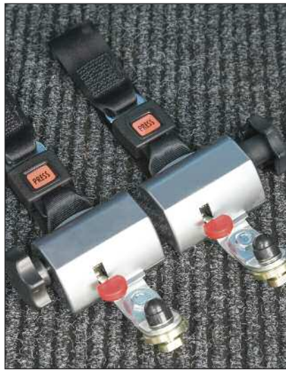
Figure 12 – Retractable rear belt with manual tensioner.
