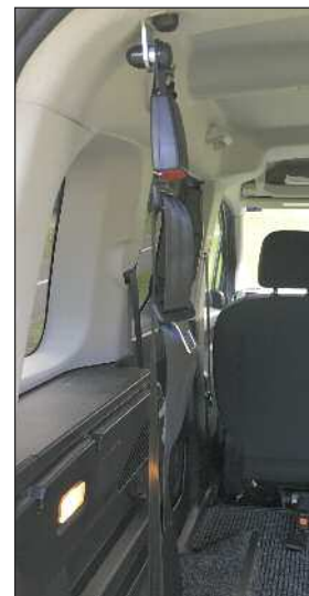
Figure 18 – Wheelchair occupant seat belt drop link height adjustment.
