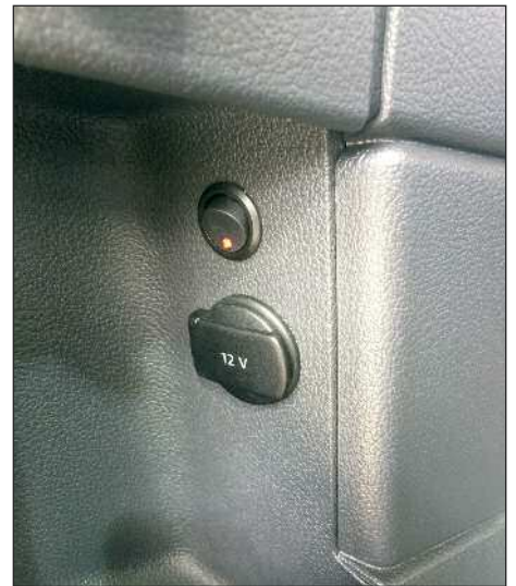
Figure 3 – Example Electric 'Inertia' Belt switch.
